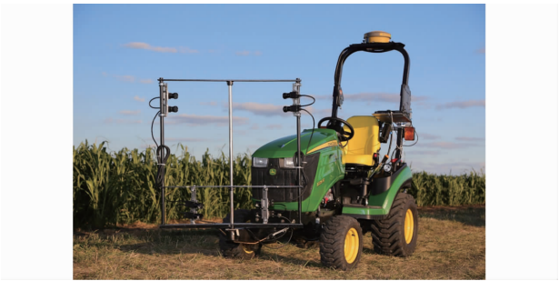
图 8 搭载在小型拖拉机上的表型平台 Fig. 8 Phenotyping platform mounted on John Deere 1026R sub-compact utility tractor
