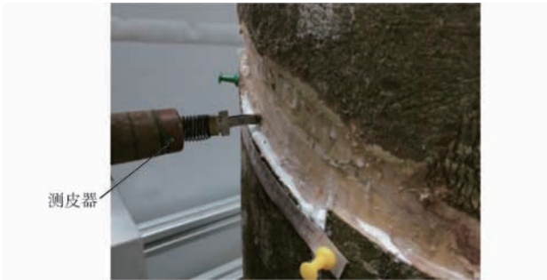
图10 割胶深度测量 Fig.10 Measurement of cutting depths
