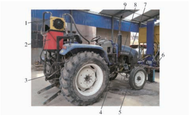
图 2 齿盘式多行拔棉秆台架 Fig.2 Dentate disc multi-row cotton-stalk uprooting bench
