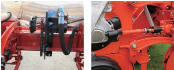
图3 液压马达驱动排种器 Fig.3 Hydraulic motor drives seed meter
