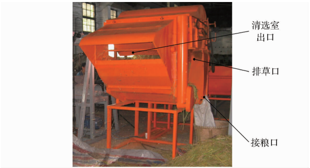
图 6 试验后物料采集区域 Fig.6 Material collecting area after experiment
