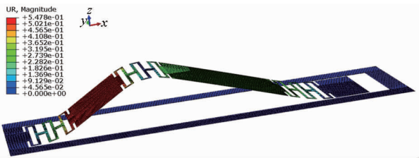
图 12 平面折展滑块机构的运行仿真图 Fig. 12 FEA model of lamina emergent slider mechanisms in operating state
