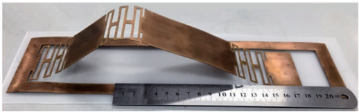
图 10 LEMs 滑块机构展开状态实物图 Fig. 10 Physical model of lamina emergent slider mechanisms in expanded state
