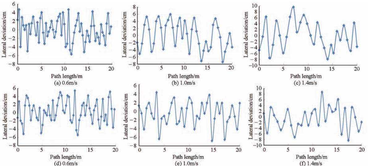
Fig. 12 Experimental results of guidance line tracking in different speed
