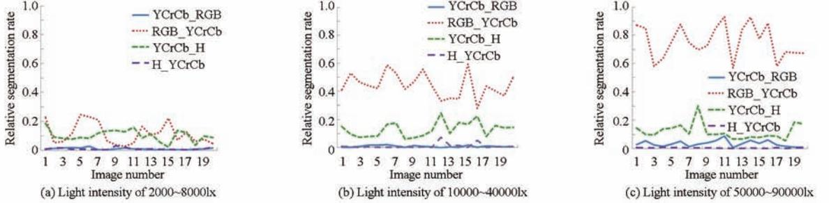
Fig. 9 Relative error curves of image segmentation under different illumination conditions
