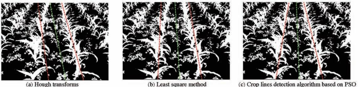
Fig. 10 Guidance line detection results of different algorithms
