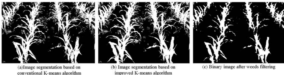
Fig. 3 Image segmentation and weed filtering
