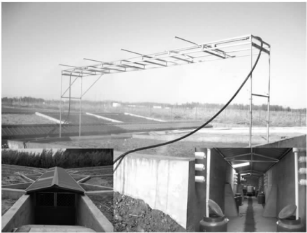
图 2 模拟降雨试验及小区结构示意图 Fig.2 Diagram of rainfall simulation experiment and structure of runoff monitoring site
