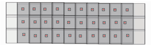
图 1 匹配中心点参与区域网平差示意图 Fig. 1 Schematic drawing of matching central point participating in block adjustment
