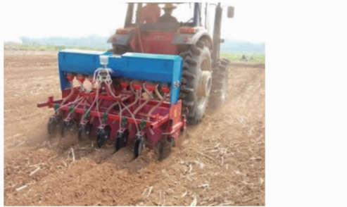
图7 枝状阀式分流装置田间播种试验 Fig. 7 Filed test of valve-branch distributor
