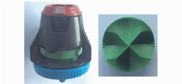
图 1 Nelson R3000 型喷头及绿色喷盘 Fig.1 Nelson R3000 sprinkler with green plates used in investigation
